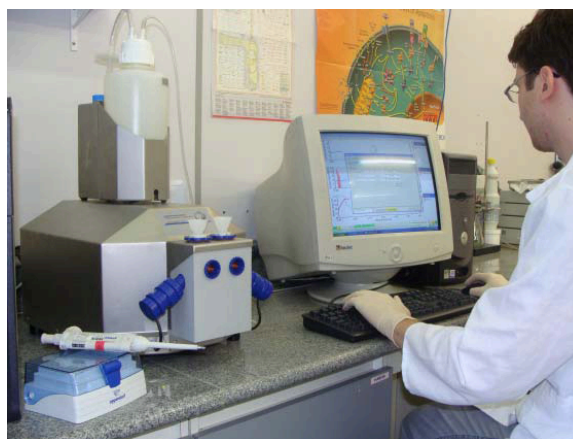
Oxygen consumption- The oxygraph is changing the sensitivity standards for monitoring oxygen consumption by cells and organelles.
