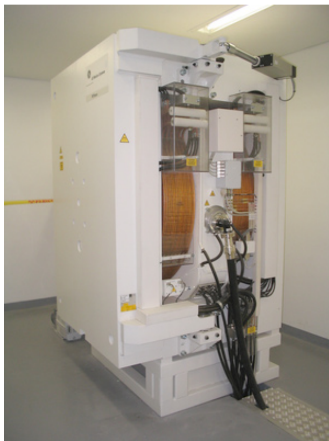
The PETtrace is an integrated system of production of PET tracers that comprise a negative ion cyclotron control system with a workstation operator, target systems and synthesis systems.
