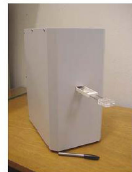
Fluorometer dedicated to the detection of luminescent markers based on rare earths ions.
