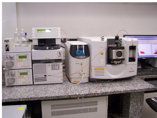
Equipment for Phenolic compounds analysis by LC-DAD-ESI-MS
